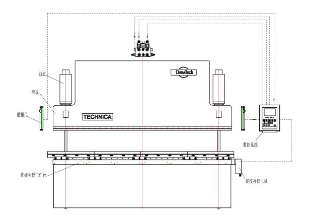
The machine is constructed by main frame, upper beam, back gauge system, sliding system, Synchronization control device, tooling, hydraulic system, CNC system etc.
