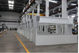
and carefully work. Machines used in high quality steel welded structure, frame is heavy style and strong rigidity, painting imported antirust primer and surface coat to make machine durably and newly. The main frame and upper beam slider are made
